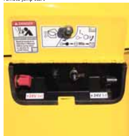
Hood opening and battery on/off switches. In case of flat battery, hood opening can be done externally with remote jump start
