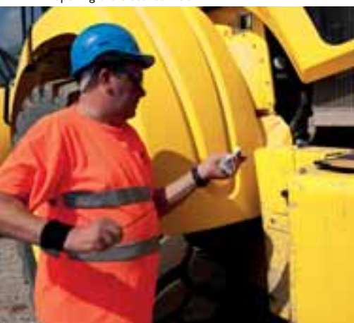
Engine oil level check can easily be performed slightly opening the electrical hood
