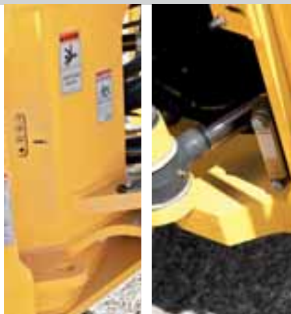
Grouped greasing points and visual transmission oil level check for easy daily maintenance
