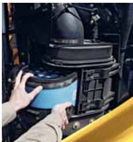
The removal of air filter can be done from ground level in a few seconds
